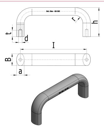
$\begin{array}{lll} a & = 17 \\ b & = 26 \\ d & = M8 \\ h & = 57 \\ I & = 500 \\ r & = 17 \\ t & = 12 \\ Weight in (g) = 538 \\ \end{array}$
